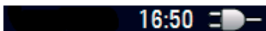
Fig.: R&S ZVH is being powered by the AC supply and the battery is fully charged
